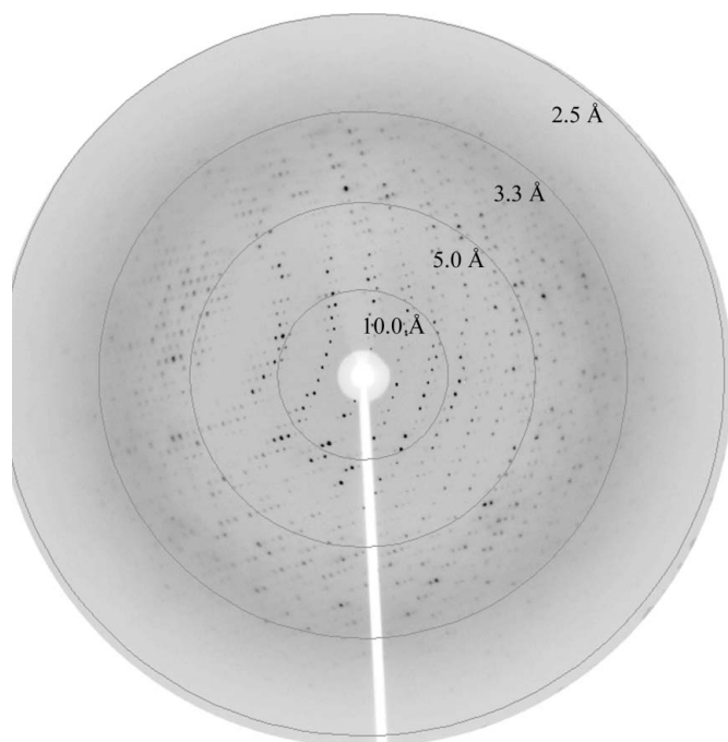
Figure 3 X-ray diffraction of an SeMet NCS crystal to 2.7 Å at the peak wavelength ( \lambda = 0.97966 Å). Data were collected as 1.0° oscillation frames at 100 K.
